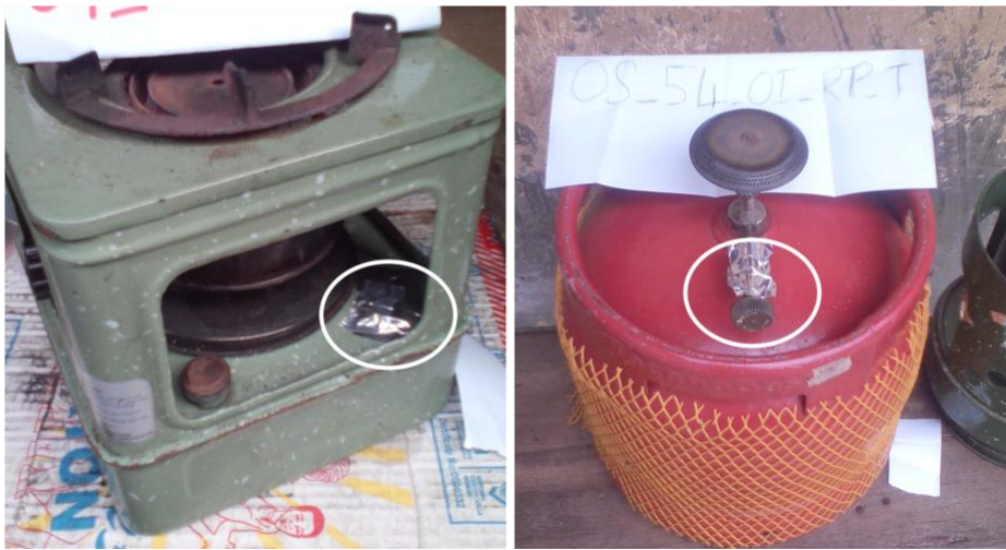
Figure 1: Kerosene stove (left) and LPG (right) fit with a SUMS iButton (model DS1922T, Maxim, USA)
